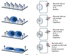
Figure 1. Impedance measurement principle in real-time monitoring using xCELLigence system
