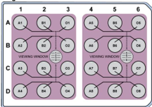
**Figure 1. BioFlux 24-well plate channels.**
