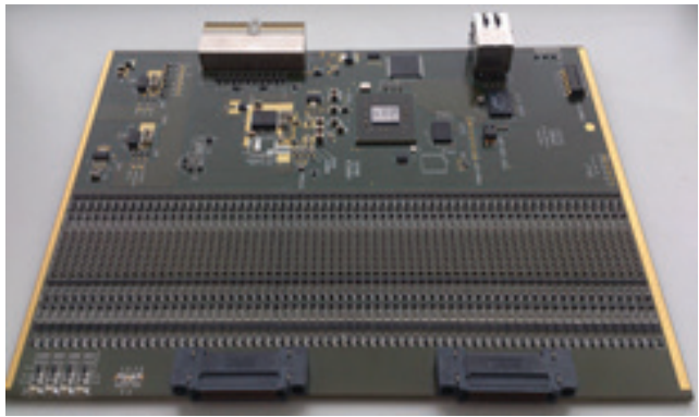
66-channel ADC board with FPGA processing capabilities. Signals are simultaneously sampled (no multiplexing). Each board digitalizes the signal from 2 PET modules. The overall DAQ system employs a 10 Gb Ethernet switch
