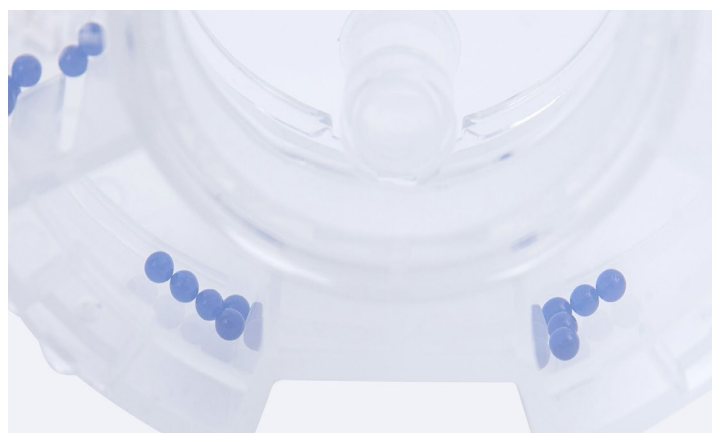
Integral humidification system with hydratable beads prevents water-loss from the culture chamber. The rest of the ClinoStar can operate at ambient humidity: this reduces the contamination risk to the cultures.
