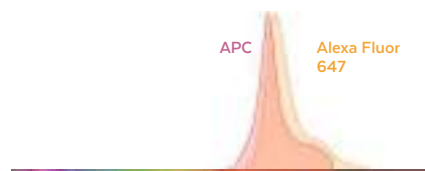
Figure 1: Spectrum plots from a conventional spectrum viewer shows heavy overlap between APC and Alexa Fluor 647.
