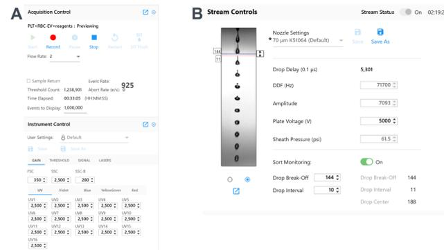
Figure 1. Cytek ESP Detection Option instrument settings (A), and 70 µm nozzle settings (B).
