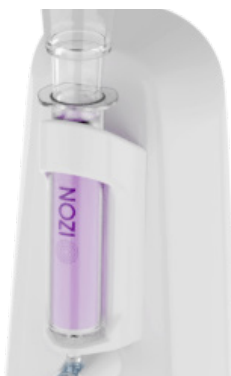
Figure 10: A qEVoriginal/70 nm Legacy column loaded correctly onto the AFC. Ensure that the Izon logo is facing away from the AFC tower.
