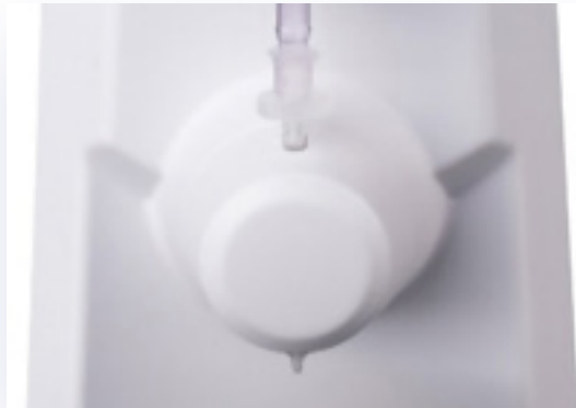
Figure 21: Pinch valve cover on.
