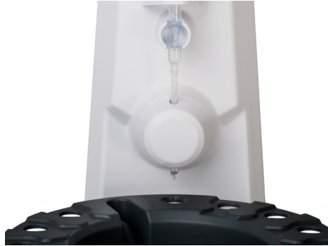
Figure 7: The nozzle tip centred over the flush hole. Note that for the side of the carousel that holds 2 mL tubes, the flush hole will be on the right of the central well channel. For the other side of the carousel that holds 5 mL tubes, the flush hole is on the left of the central well channel.
