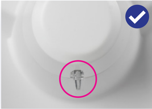
Figure 26: Nozzle tip fully emerging through the hole in the pinch valve cover.
