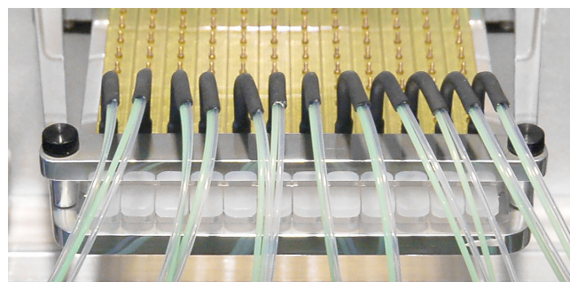
12 ingredient inputs with tubing that can be used with any virtually any container
