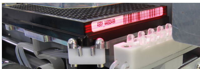
optional barcode scanner automatically loads and executes dispenses
