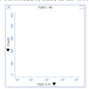
3.1.3 Buffer Control Group: Place the sample buffer (e.g., PBS buffer) into the sample rack and click the **Start** button. Set the P1 gate in the acquired histogram to exclude the instrument's background noise. Calculate the product of the EPS and the percentage of events within the P1 gate (EPS × P1 percentage). If this value is below 50, it indicates that the buffer background meets the requirements and can be used for subsequent experiments.
