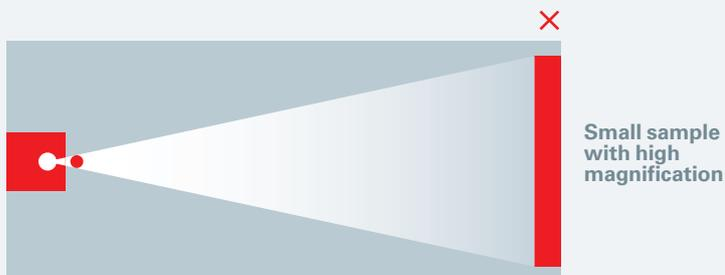
Conventional fixed camera systems are limited to one scanning speed, regardless of the sample size or magnification.
