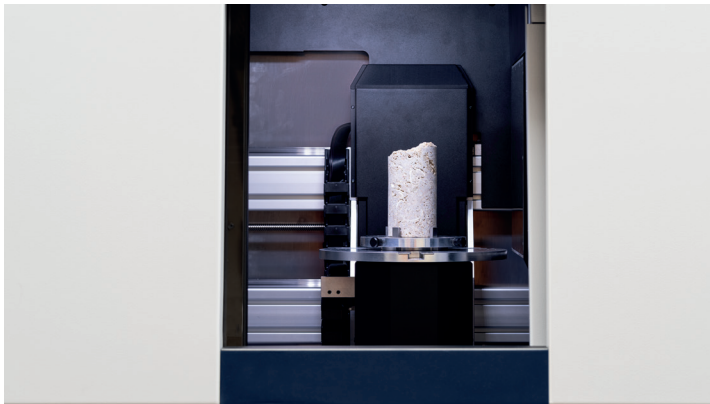
Large chamber for mounting big samples and optional sample stages
