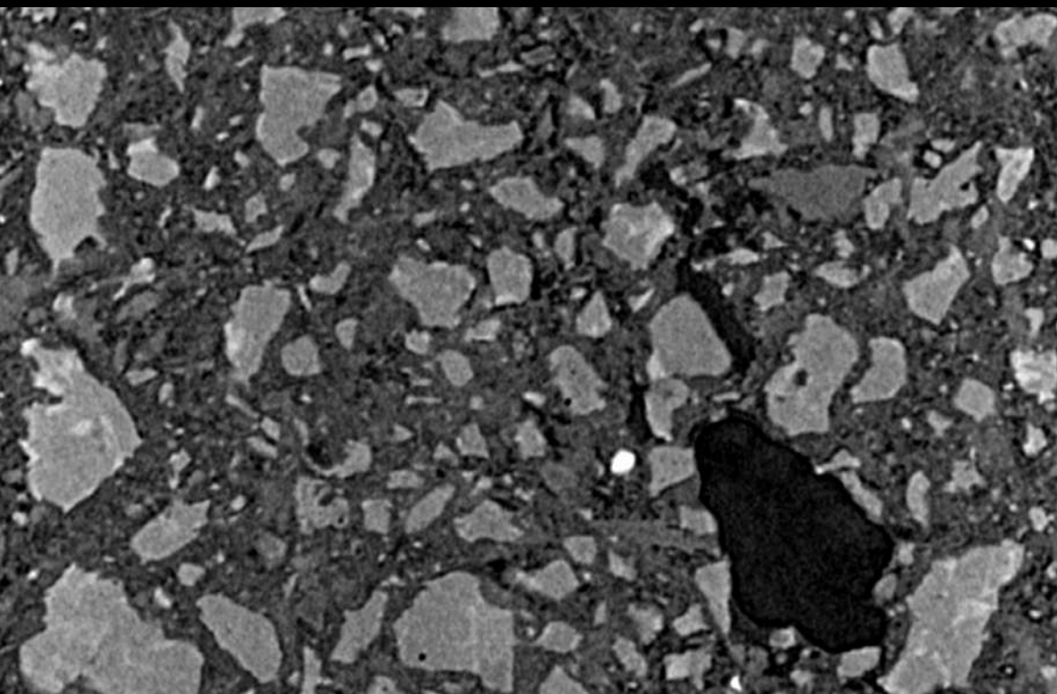
Hydrated cement in capillary scanned at 220 nm.
